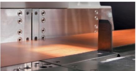
Perfect alignment of very thin and/or flexible panels, minimising cycle times thanks to the **side alignment stop** integrated in the blade carriage.
